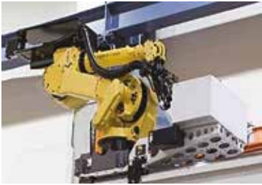
The tool exchange can be performed between machines as well by Interchanging the tools between the tool room and the machines.
